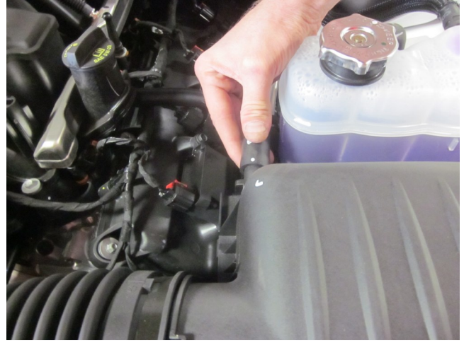
d) Unhook the valve cover breather tube from the stock air box.
