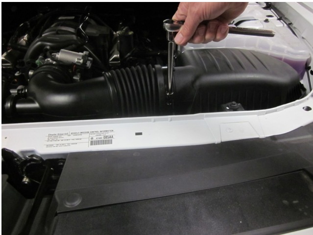
a) Loosen the hose clamp that connects the intake tube to the stock air box.
