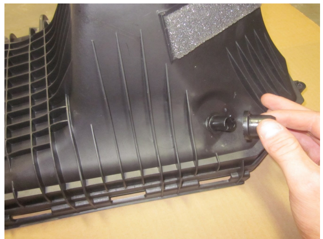
f) Remove the rubber sleeve on the stock air box and place it to the side to be reused later in the installation.
