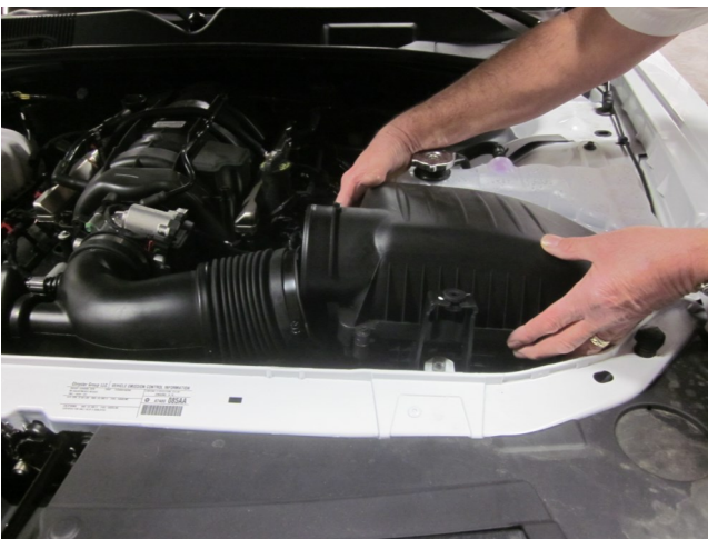
e) Remove the complete stock air box by pulling up and out of the vehicle.
