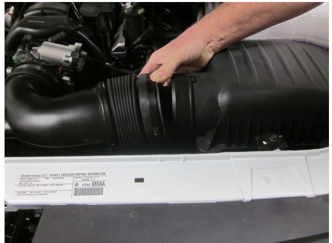
b) Disconnect the intake tube from the stock air box.
